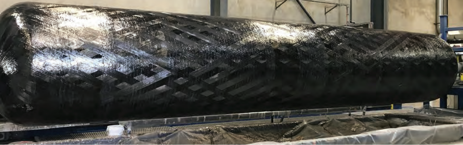
Large carbon fibre composite pressure vessel constructed using Omni Tankers OmniBIND technology
